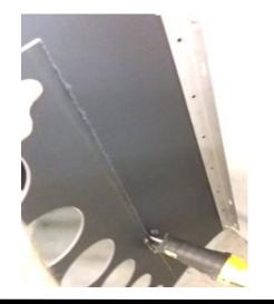
14) Attach dissipator to bracket with screws. Adjust your drill's torque setting to prevent stripping. Repeat Steps 12—14 at other bracket.
