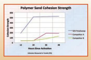
**COHESION** PolySweep achieves superior cohesion versus the competition by a factor of 6 (180 psi VS 30 psi) within 12 hours of activation. PolySweep maintains superior cohesion performance at 24, 36, and 48 hours after activation. (See chart.)
