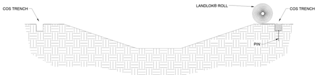
Figure 10: Crest of Slope (COS) Trench Placement
