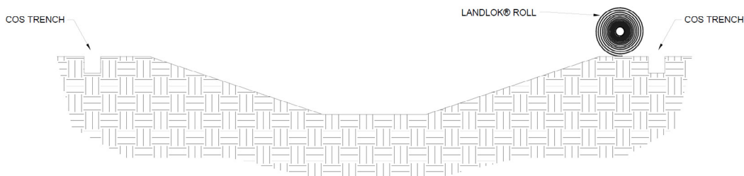
Figure 9: Crest of Slope (COS) Trench Alignment
