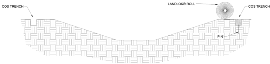
Figure 10: Crest of Slope (COS) Trench Placement
