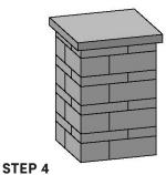
Place a column cap to finish the pillar. The column cap can be cored as needed for installation of a light.
